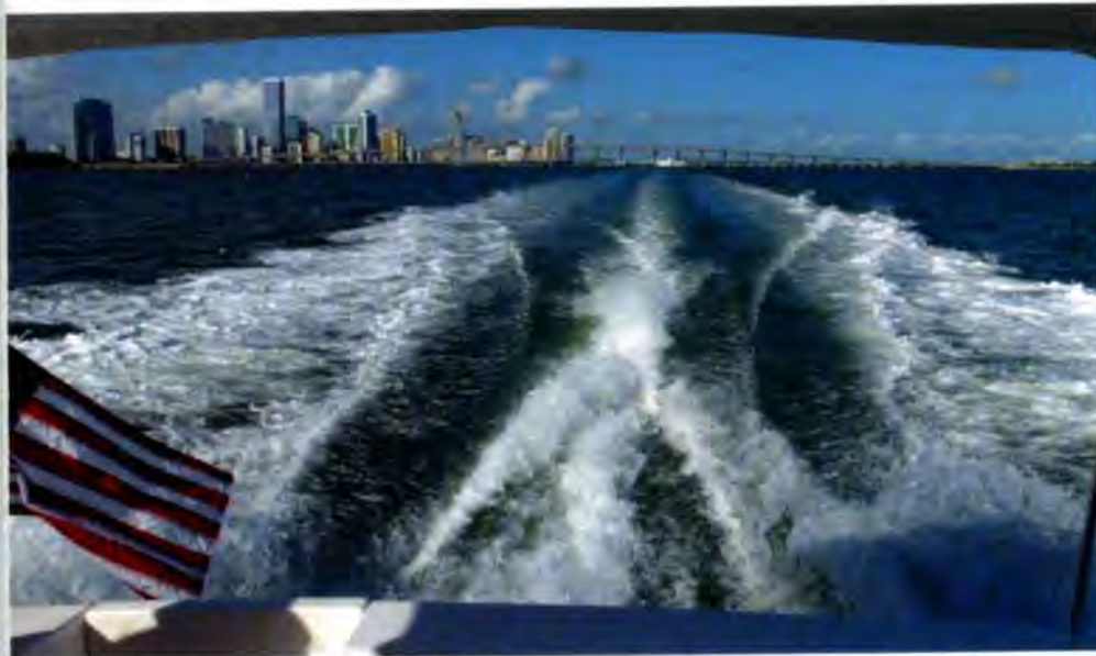
Opposite: The SRD reverse deadrise stern can be clearly seen on a boat under construction. Above: This slippery shape results in almost no wake running at 17 knots.
